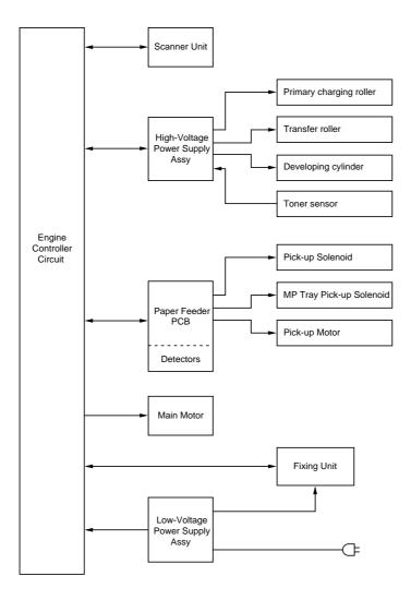
Figure 3.5 Engine Controller Block Diagram
