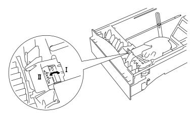
Fig. 2-15 Switching the Adjustment lever by Paper Size
