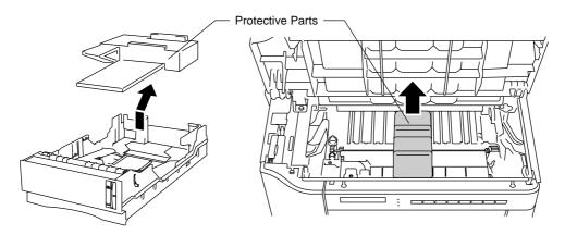
Fig. 2-7 Removing the Protective Parts
