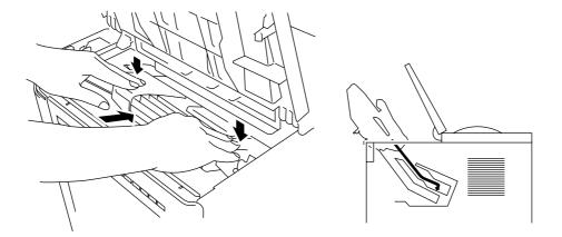
Fig. 2-13 Inserting the Toner Cartridge
