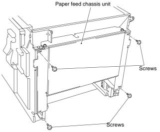
Note: When installing the paper feed chassis unit, screw the left chassis of this paper feed chassis unit, set the paper tray, displace the right chassis of this unit up to the paper tray and screw them.
