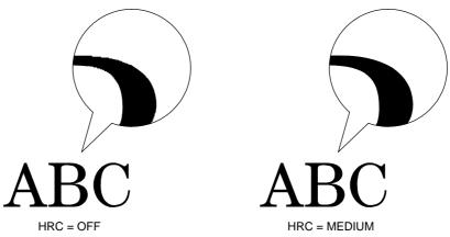
Fig. 4-5 High Resolution Control
