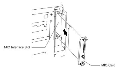
Fig. 5-4 Installing the MIO Card
