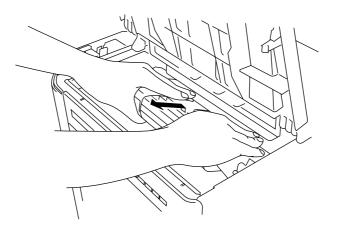
Fig. 7-9 Removing the Toner Cartridge
