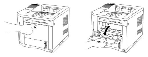
Fig. 2-19 Opening the Multi-purpose Tray and Pulling Out the Extension Tray
