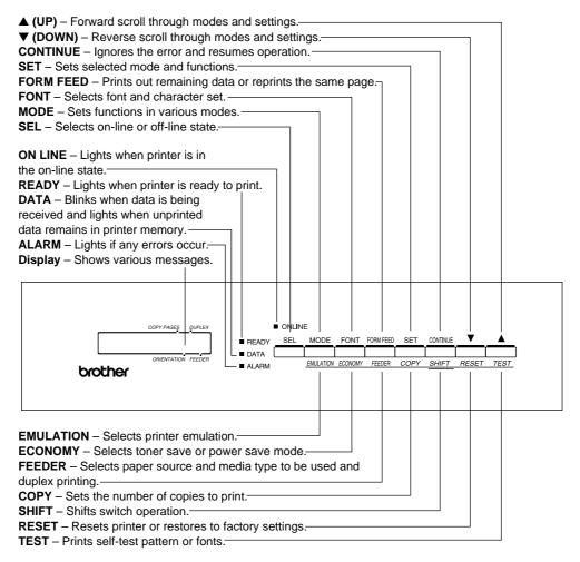
Fig. 3-2 Switch Operation in NORMAL and SHIFT Modes
