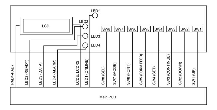
Figure 3.8 Display Circuit
