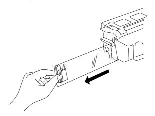
Fig. 2-12 Pulling Out the Sealing Tape
