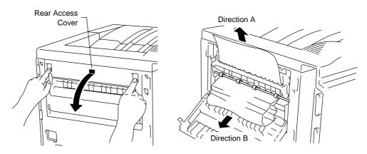
Fig. 7-3 Paper Jam at Rear Access Cover
