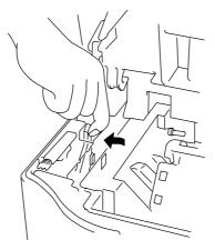
Fig. 5-5 Unlocking the Left Side Cover
