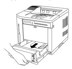
Fig. 2-14 Removing the Paper Cassette
