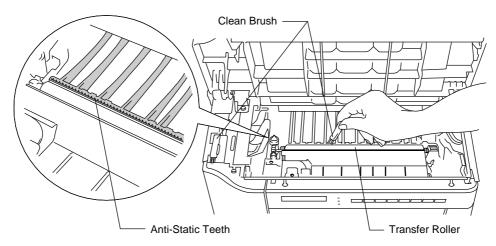
Fig. 6-1 Cleaning the Anti-Static Teeth
