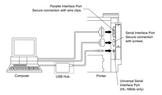
Fig. 2-21 Connecting the Printer and Computer
