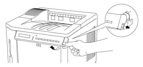
Fig. 3-1 Adjusting the Control Panel Angle
