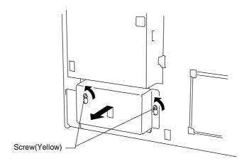
Fig. 5-7 Removing the Metal Cover
