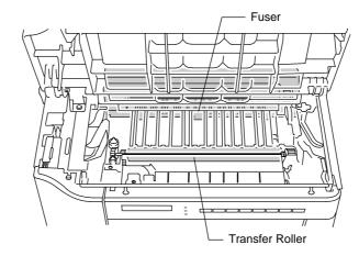
Fig. 6-5 Fuser and Transfer Roller
