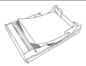
Fig. 2-18 Loading Paper into the Cassette
