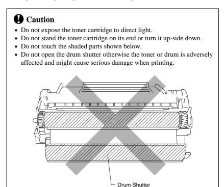
Fig. 2-9 Don'ts When Handling the Toner Cartridge
