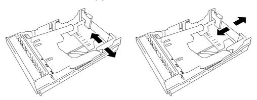
Fig. 2-17 Adjusting the Paper Cassette Sizes
