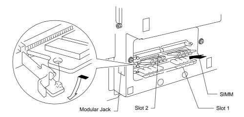
Fig. 5-8 Installing the SIMMs
