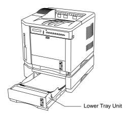
Fig. 5-1 Loading Paper in the Lower Tray Unit
