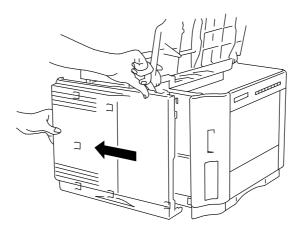
Fig. 5-6 Removing the Left Side Cover
