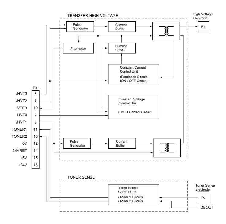
Figure 3.11 High-Voltage Power Supply Block Diagram 2
