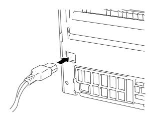
Fig. 2-22 Plugging in the Power Cord
