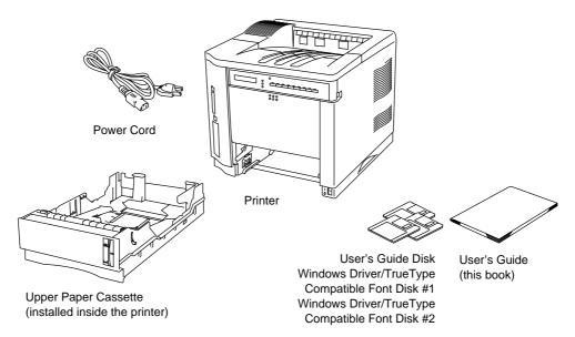
Fig. 2-1 Components in the Printer Carton
