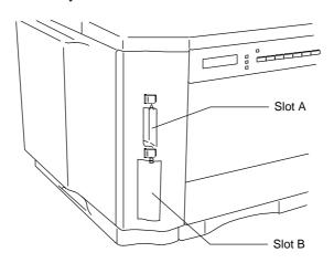
Fig. 5-2 Installing or Removing the Cartridge or Card
