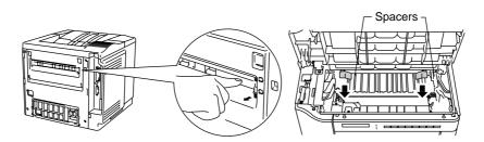
Fig. 2-7 Removing the Protective Parts
