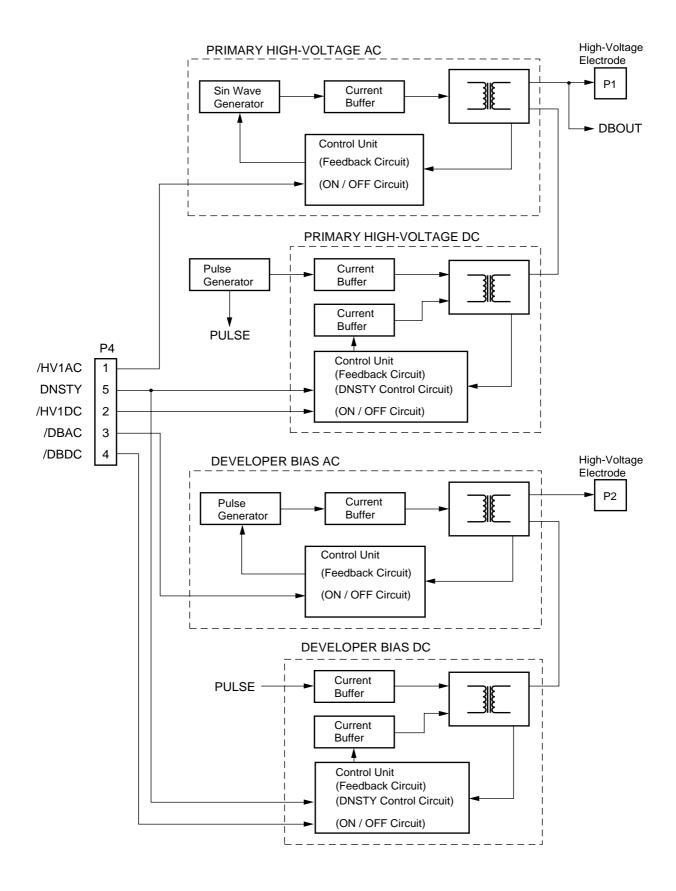
Figure 3.10 High-Voltage Power Supply Block Diagram 1
