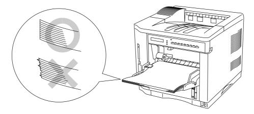
Fig. 2-20 Placing Paper on the Multi-purpose Tray
