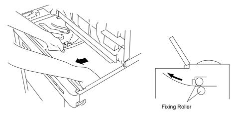
Fig. 7-4 Paper Jam at Fixing Roller
