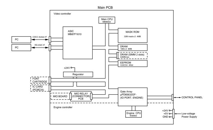
Figure 3.1 Main PCB Block Diagram
