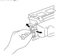
Fig. 2-11 Detaching the Tab
