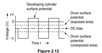
An AC bias is applied to the developing cylinder to help project the toner particles to the drum surface and improve the contrast of the printed image. The center voltage of the AC bias (1600 Vp-p) varies with the DC bias voltage.
