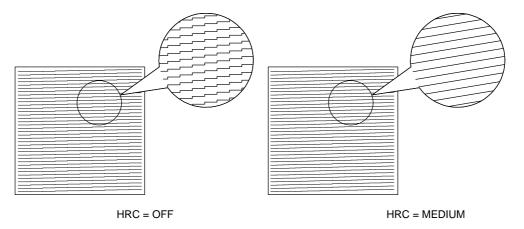
Fig. 4-6 High Resolution Control in Test Printout
